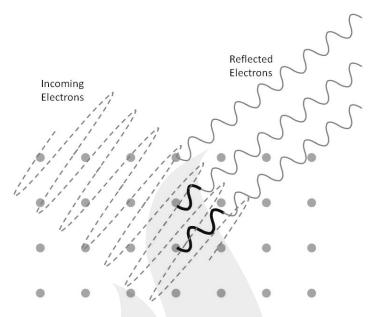
Diffraction of electrons off a crystal of nickel. An incoming electron beam (dashed line) passes into a regular crystal of atoms, and bits of the wave (individual electrons) reflect off different atoms in the crystal. Electrons reflected from deeper in the crystal travel a longer distance on the way out (darker line), but for certain angles, that distance is a multiple of a full wavelength, and the waves leaving the crystal add in phase to give the bright spot seen by Davisson and Germer.
