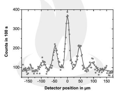
The interference pattern produced by a beam of molecules passing through an array of narrow slits. The extra lumps to either side of the central peak are the result of diffraction and interference of the molecules passing through the slits. (Reprinted with permission from O. Nairz, M. Arndt, and A. Zeilinger, Am. J. Phys. 71, 319 [2003]. Copyright 2003, American Association of Physics Teachers.)
