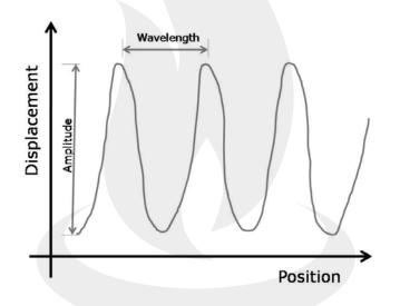
As you move along the pattern, you see the medium moving up and down by an amount called the "amplitude" of the wave. If you measure the distance between two neighboring crests of the wave (or two troughs), you've measured the "wavelength," which is one of the numbers used to describe a wave.
