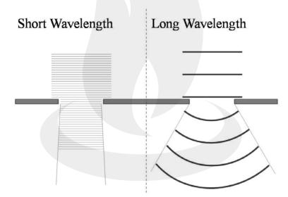
On the left, a wave with a short wavelength encounters an opening much larger than the wavelength, and the waves continue more or less straight through. On the right, a wave with a long wavelength encounters an opening comparable to the wavelength, and the waves diffract through a large range of directions.
